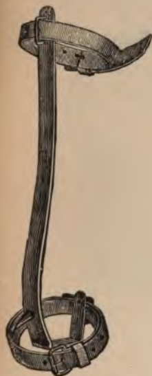
FIGS. 232-233.—Eastern pole climbers, with and without strap for attaching to legs.
